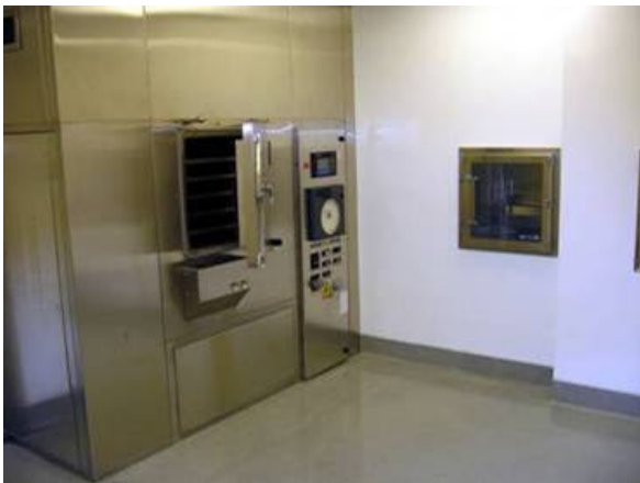
This depyrogenation oven, which is required as part of GMP regulations, uses dry heat at extremely high temperatures to burn off contaminants and proteins from glassware and glass vials. (Photo courtesy of St. Jude Children's Research Hospital.)
